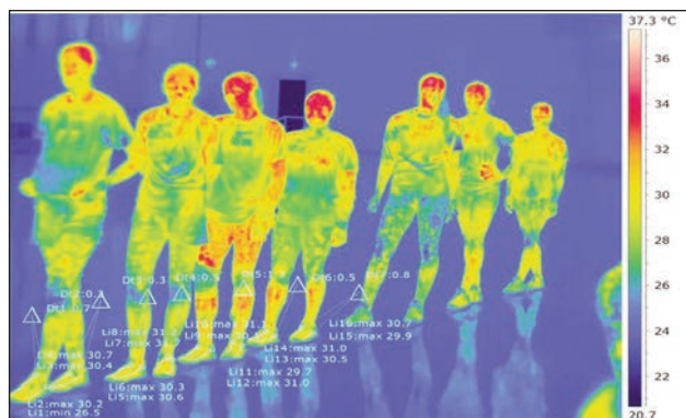
Fig. 10. Variation of sports footwear type A temperature at time three on the 4 subjects in infrared
