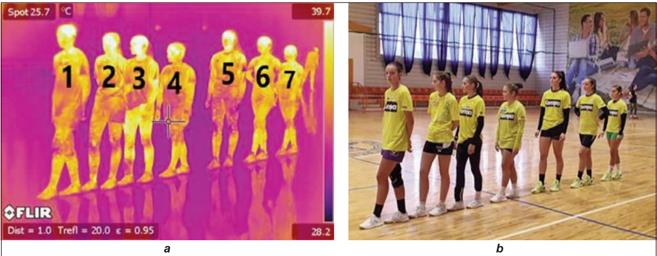
Fig. 2. IR and real spectrum image of the seven subjects: a – infrared image; b – real image
